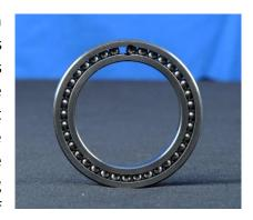
When using AMB to support a rotating shaft, any reduction or loss of power could cause the shaft to drop. With an NES AMB back-up bearing in place, the shaft will drop onto the back-up bearing system, allowing the shaft to coast to a stop without causing damage to the shaft or surrounding machinery.
